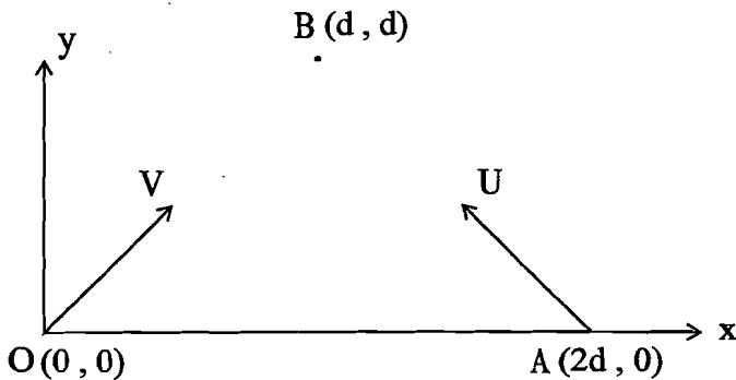
Two projectiles are projected at the same time towards a target at point B(d,d). One of the projectiles is projected from O(0,0) with a velocity V, while the second projectile is projected from A(2d,0) with velocity U.
